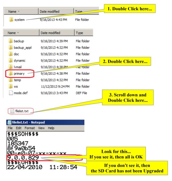
If it is OK, then take SD Card out of the card reader and put it into the IP Office. It will keep the original Feature Key number but it will be a Release 9.0 SD Card. If the SD Card did not upgrade, do not put it in the KSU.
